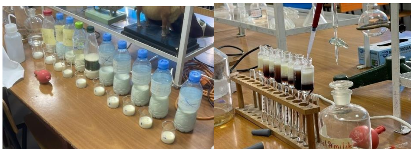
Figure 3 a), b): Filling the butyrometers with milk, adding acid (a), adding alcohol (b)
