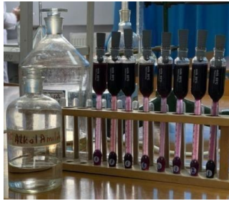
Figure 4 a), b): Images of the process of burning chemical components of milk except fat
